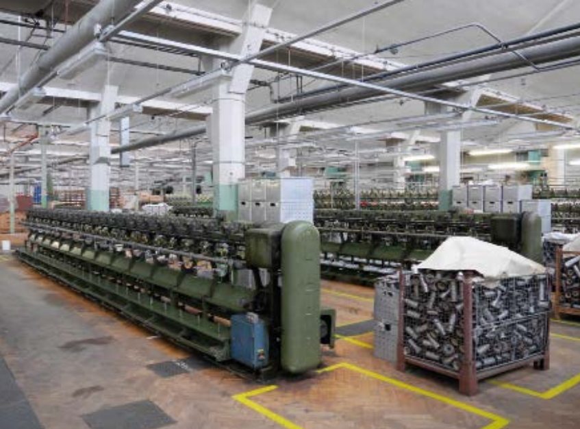
Šumperk, V. Vinciguerra & Cie., silk thread spinning mill / Hedva, Ratti plying and winding machine. Photograph by Michaela Ryšková, 2020.
