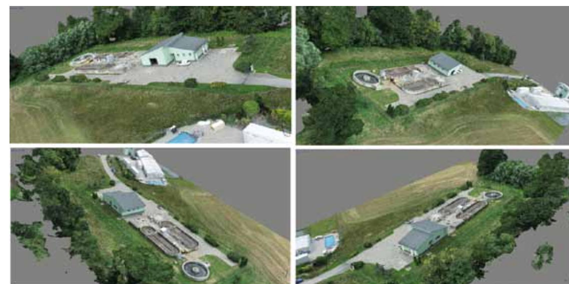
Fig. 4.271: Various displays of the 3D tiled model of a WWTP. Radek Bachan, 2021.
