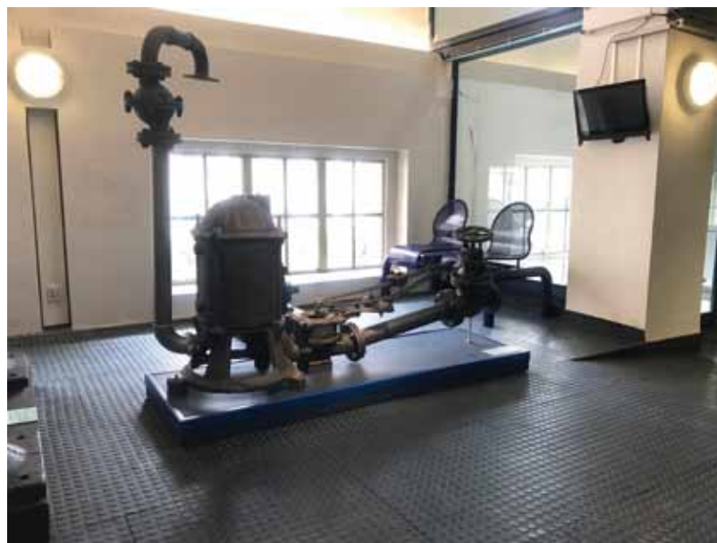
Fig. 4.201: Nové Dvory near Kutná Hora – hydraulic ram (pump based on the use of kinetic energy of flowing water) which replaced the original pump powered by a waterwheel probably in 1897. Up to the mid-1950s it supplied a manor and local chateau with non-potable water. The water source was a local pond, water was pushed to an elevated water tower, from where it flowed to its place of use. In the 1990s the pond was sold, the tank and half-timbered service house ended up in a desolate state and the hydraulic ram was forgotten. It was discovered, picked up and overhauled between 2014–2016 (Nové Dvory). Installed in the Prague Waterworks Museum (Muzeum pražského vodárenství). Photograph from the PVK archive.
