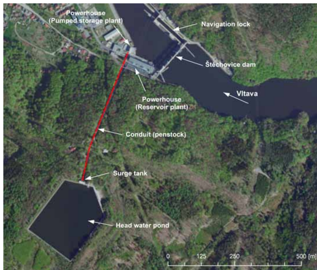
Fig. 4.138: Situation of the Štěchovice HS with a PSHPP and a HPP situated below the dam. Diagram created on the basis of the ČÚZK data, 2021.
