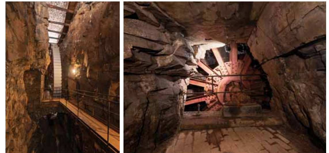
Fig. 4.166: Příbram, the Drkolnov mine – water wheel 12.4 m in diameter. Photograph by Viktor Mácha, 2019.
