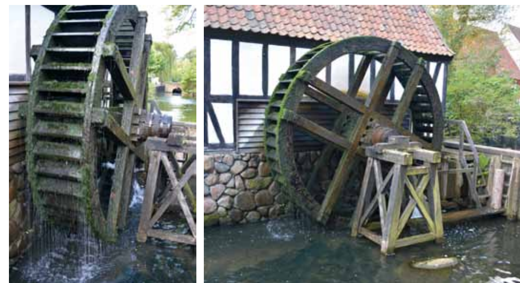
Fig. 4.168: Aarhus (Denmark), Den Gamle By – undershot water wheel with floats and shrouds, but without sole boards, which has incomplete buckets. Photograph by Radim Urbánek, 2015.
